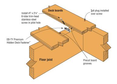
EB-TY Premium™ provides a unique method of fastening deck boards that leaves the fasteners virtually invisible. Fastening is done into the side of the board, leaving a clean, fastener-free deck surface. Apply construction adhesive to the joist for each deck board before installing the screw.
